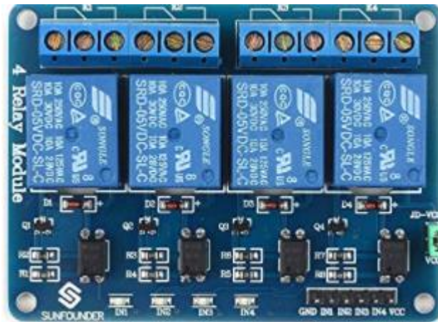
Figure 8.5: 4-channel relay module [28].
