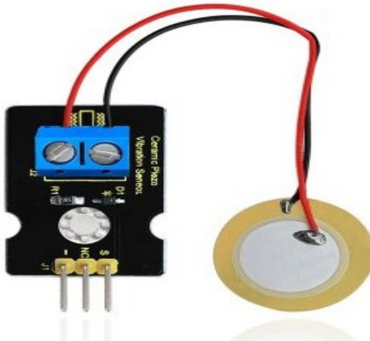
Figure 2.1 Piezoelectric Ceramic with Sensor [4]
