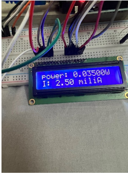
Figure 6.5 After putting 1 step, Power: 0.035W and Current: 2.5 mA
