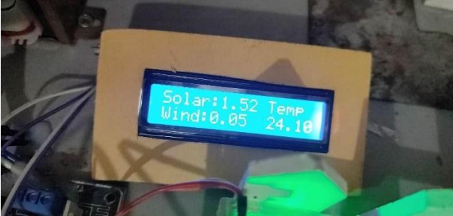
Fig: Solar and wind turbine changing Power reading of the Hardware prototype model.
