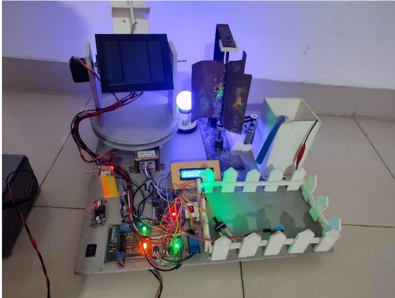
Fig: Whole Hardware model of the Wind and Double Axis 360 Degree Solar Automatic Irrigation.
