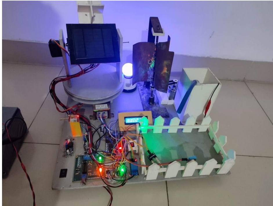
Fig: Hardware model of the Wind And Double Axis 360 Degree Solar Automatic Irrigation.
