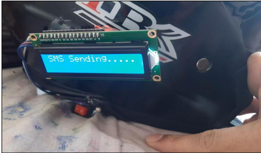
Figure 5.8: SMS Sending with live GPS location.
