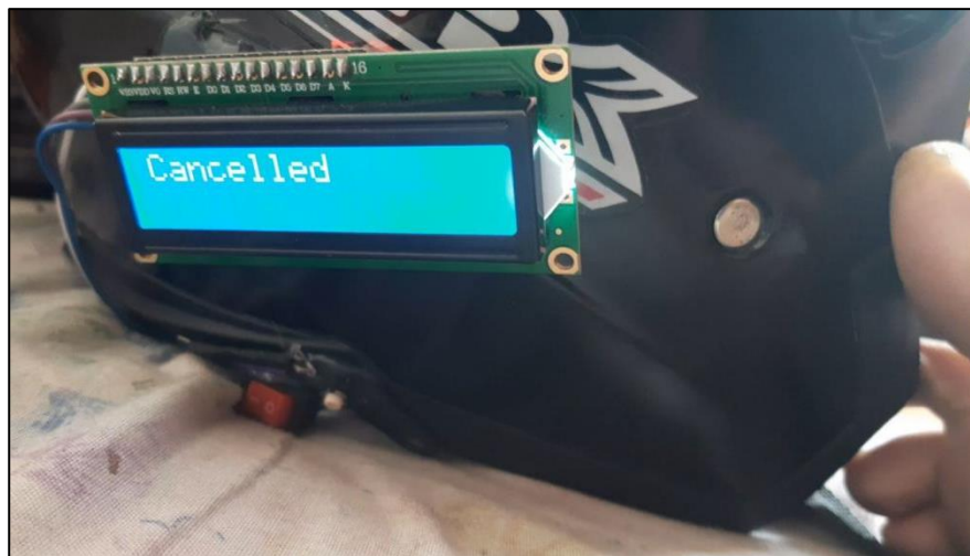
Figure 5.7: False accident alert cancelled after pressing the push button.
