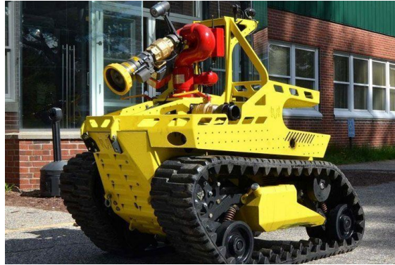
Fig 1.4: Fire Rob firefighting robots [9]
