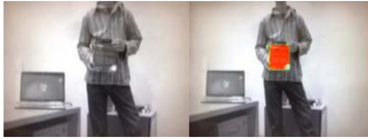
FIGURE 1.2: Color detection with tracking results: a. Image original; b. Image with a red book detected.
