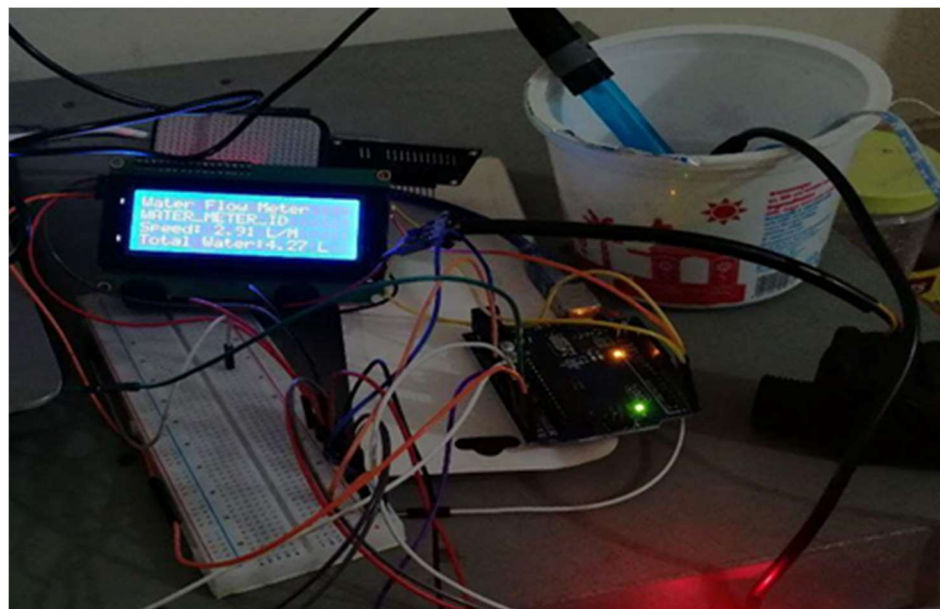
Figure 5.1 Hardware result (Water flow detection, pH measuring, Turbidity value, TDS detection).
