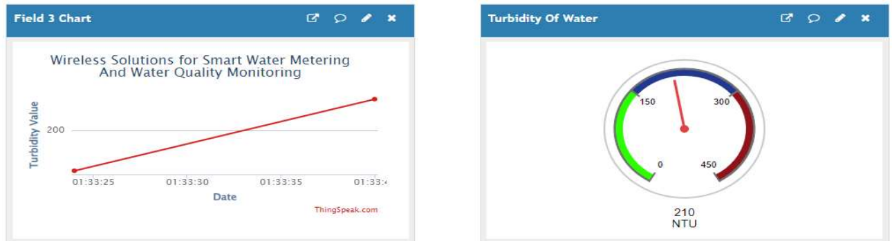
Figure 5.4 Simulated result (output result and cloud data result of turbidity value through the Turbidity sensor)
