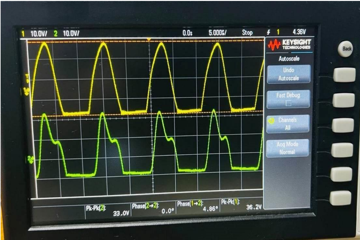
Figure 5.2: Both transmitting and receiving signal of coil for best case scenario
