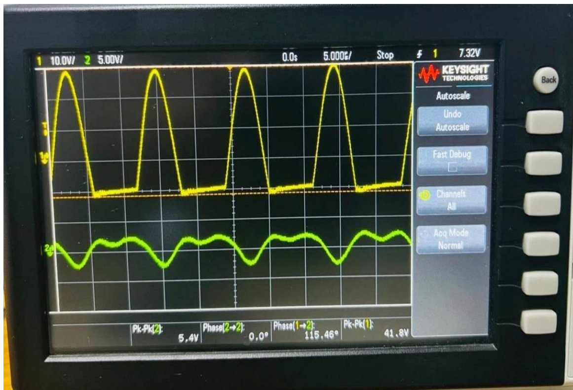
Figure 5.4: Both transmitting and receiving signal of coil for worst case scenario
