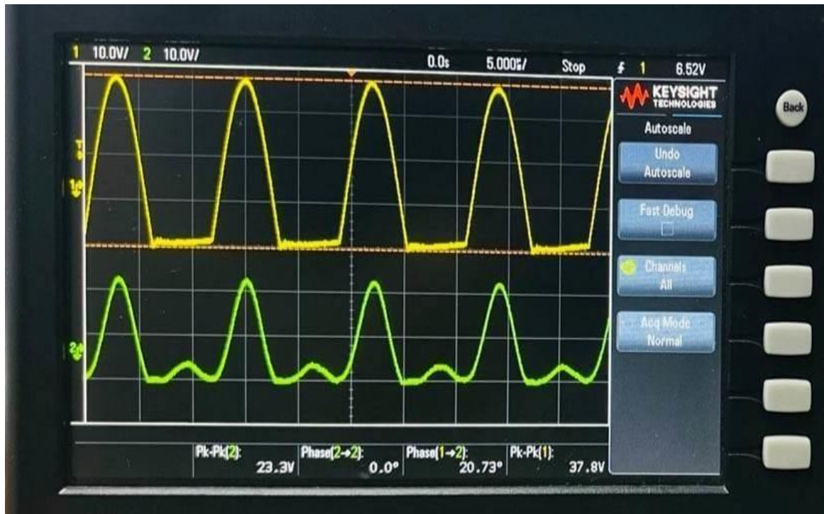
Figure 5.3: Both transmitting and receiving signal of coil for mid case scenario
