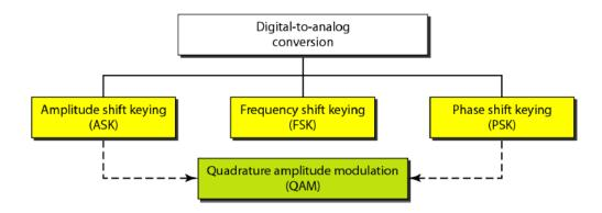
ASK: In amplitude shift keying, the amplitude of the carrier signal is varied to create signal elements Both frequency and phase remain constant while the amplitude changes.
