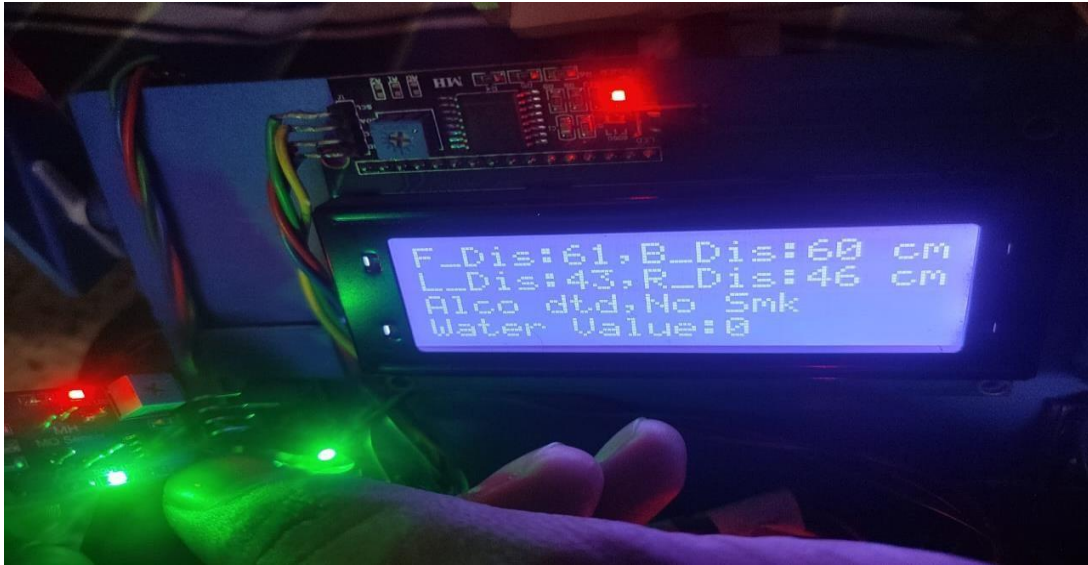
Figure 5.2: LCD Display Showing Location with No Alcohol and No Smoke Result
