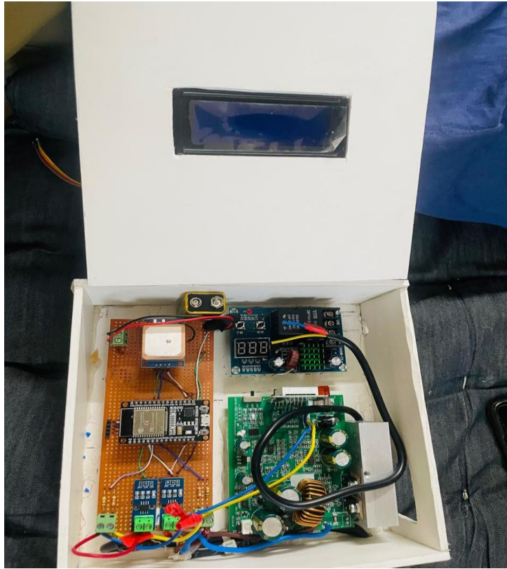
Figure 4.8: MPPT (Maximum Power Point Tracking) Charge Controller
