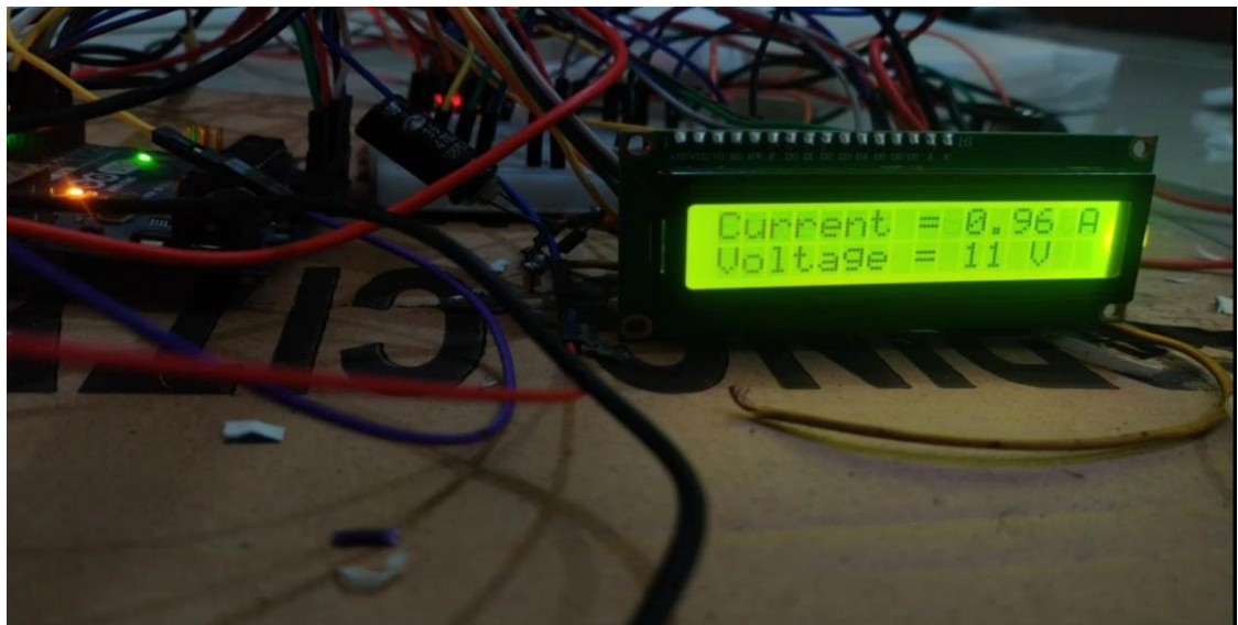
Figure 5.4: Output voltage and current under high light condition
