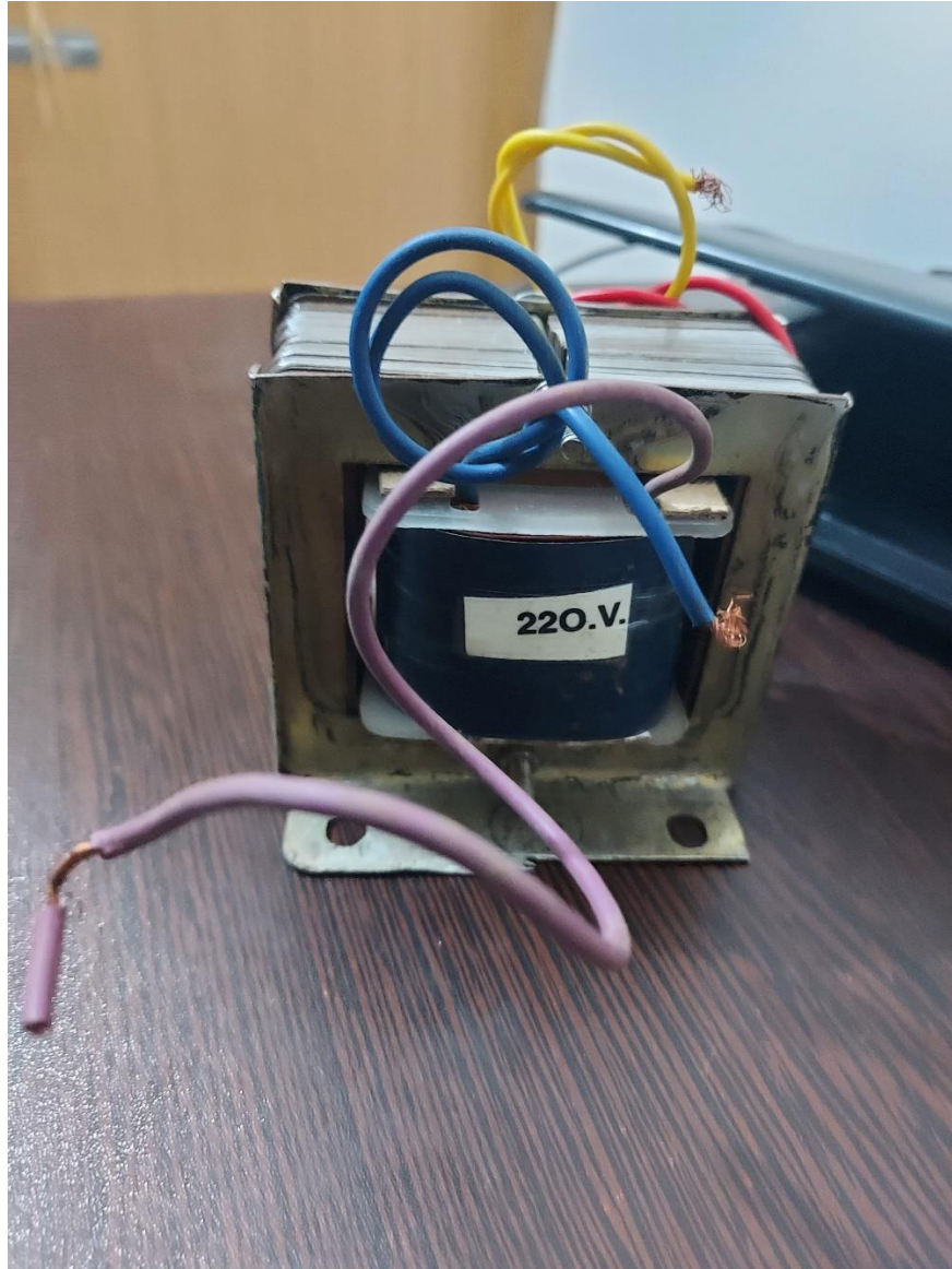
Figure 4.5 Step – Down Transformer
