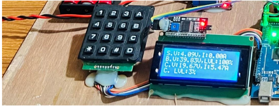
Figure 4.3.13 Charging from Solar battery
