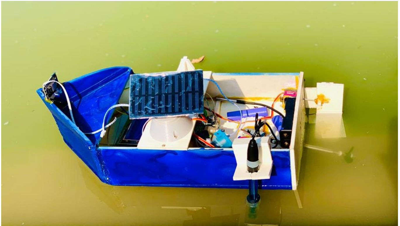
Figure 4.18: Full Hardware Structure
