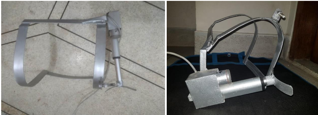
Figure: 12 construction of the metal frame for upper hand
