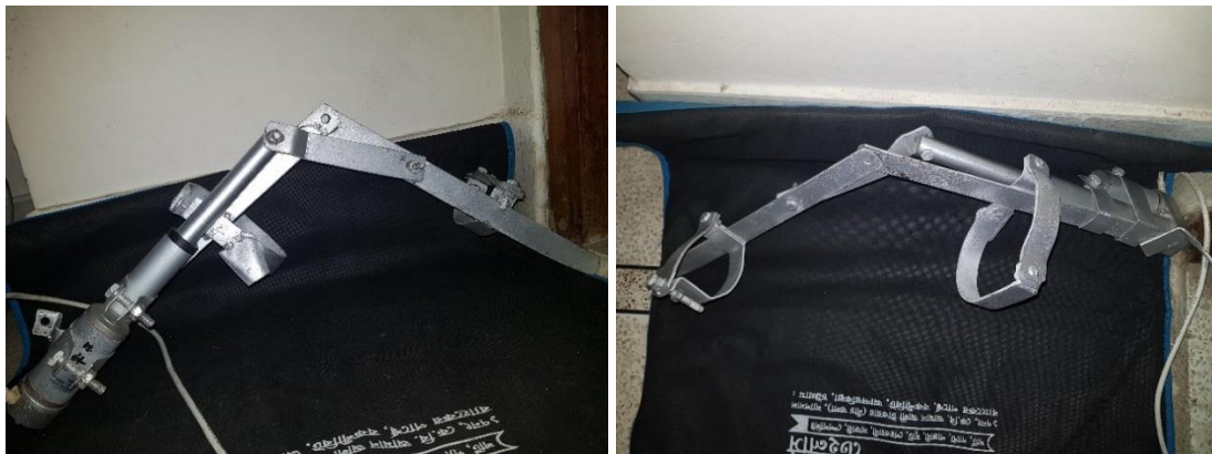
Figure: 11 construction of the metal frame for Elbow
