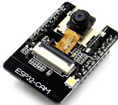
Figure 4. 14 SP32-CAM Wi-Fi + Bluetooth Camera Module Development Board ESP32 with Camera Module OV2640 [20]
