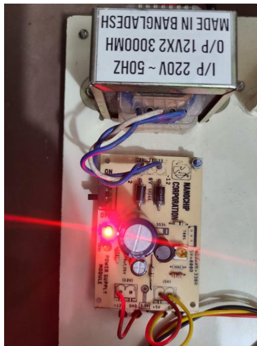
Figure 5.12: Power supply unite
