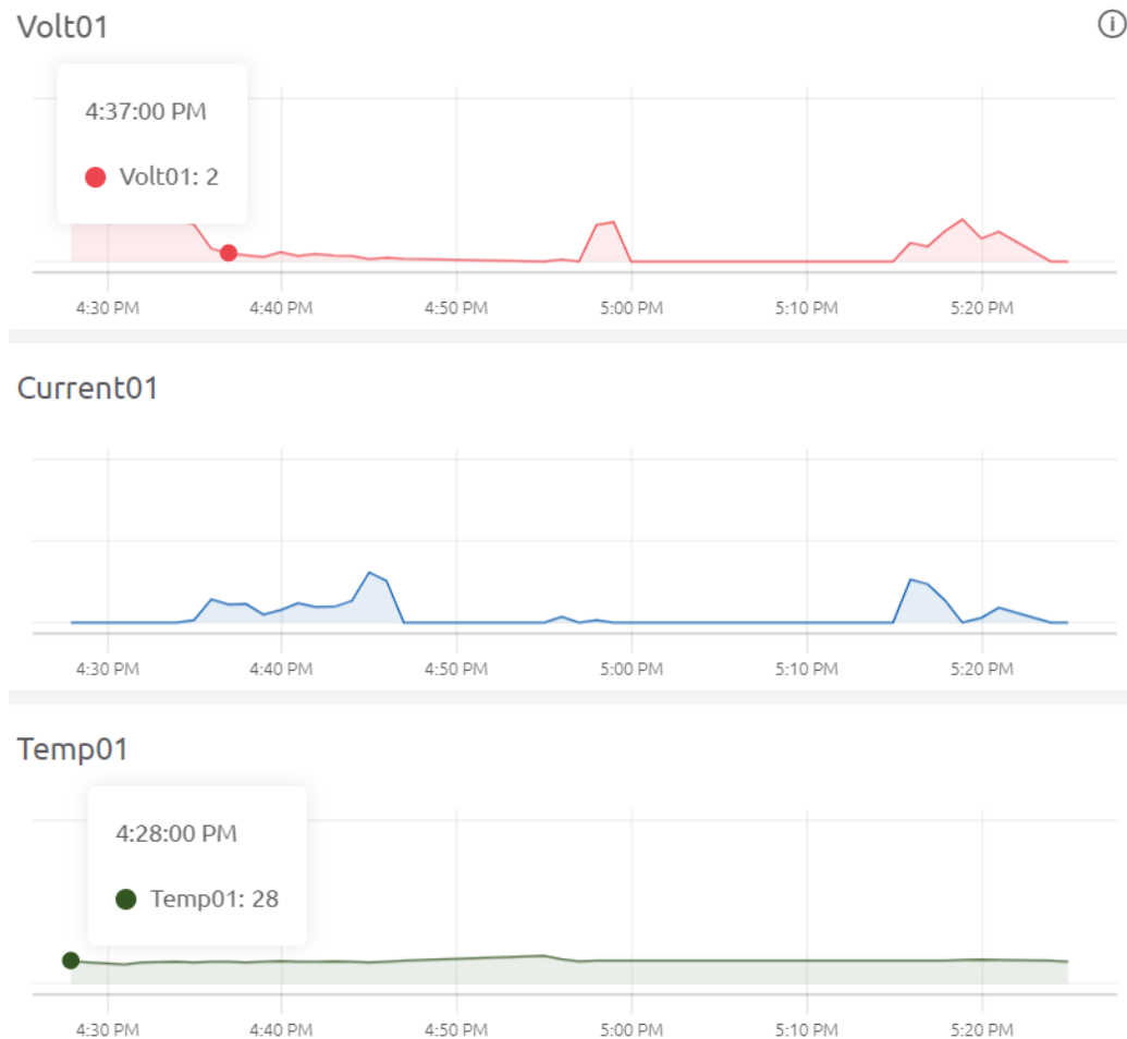
Figure 5.1: Transformer-1 Monitoring Data from IoT module with current, voltage and temperature.
