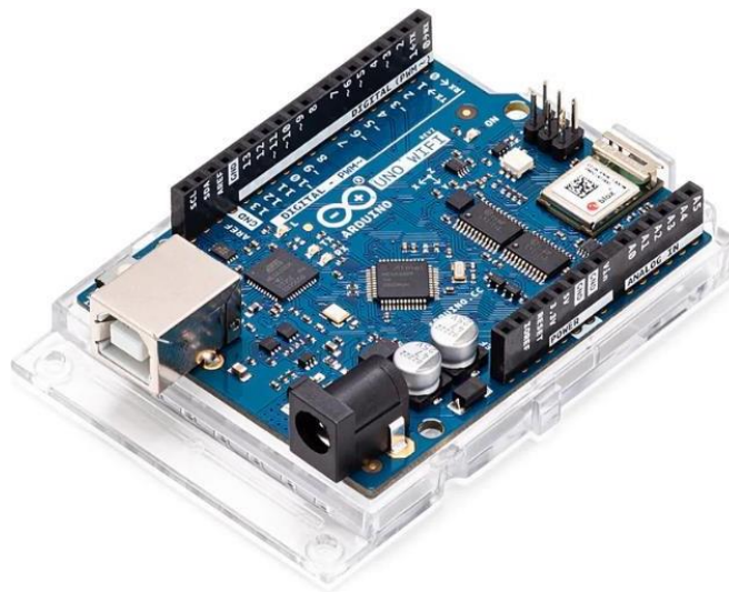
Figure 4.5: Arduino Uno Hard ware Image
